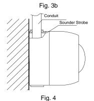
If the sounder strobe is required to be tamper-proof, knock down the arch knockout as shown in Fig. 1 and fix it with ST2.9×6.5 self- tapping screws (in this case, it can only be removed by a cross screwdriver).
